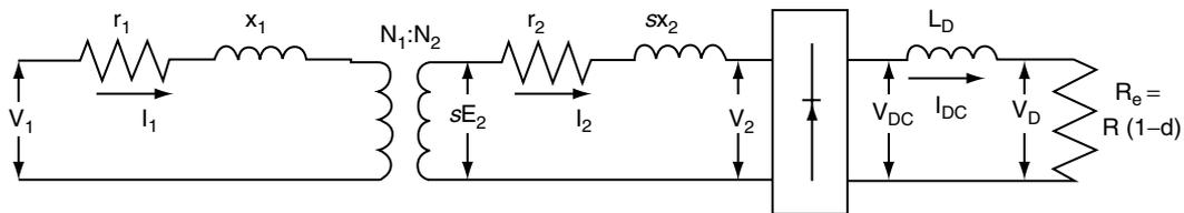
Figure 4: Equivalent circuit of a WRIG.
