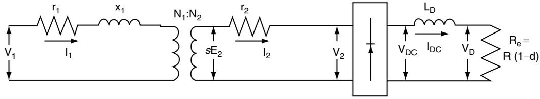
Figure 5: Approximate equivalent circuit of a WRIG.
