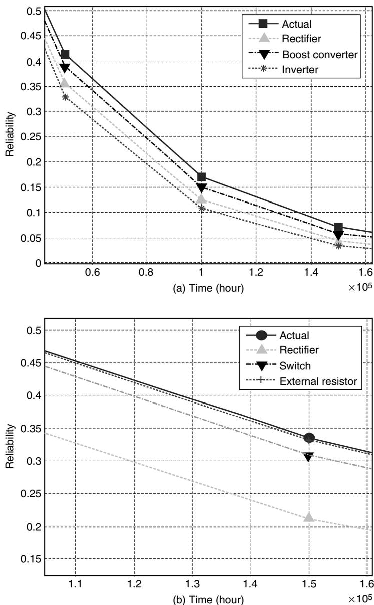
Figure 10: Effect of reliability variation of the components for a) PMG-based system, b) WRIG-based system.
