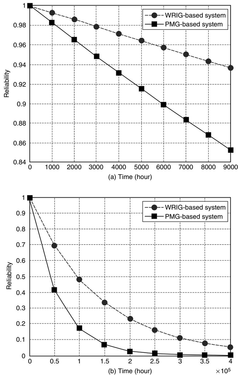
Figure 9: Reliability of the power conditioning system a) Over a year, b) Over time.
