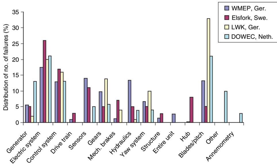
Figure 3: Distribution of number of failures of small wind turbine subsystems.
