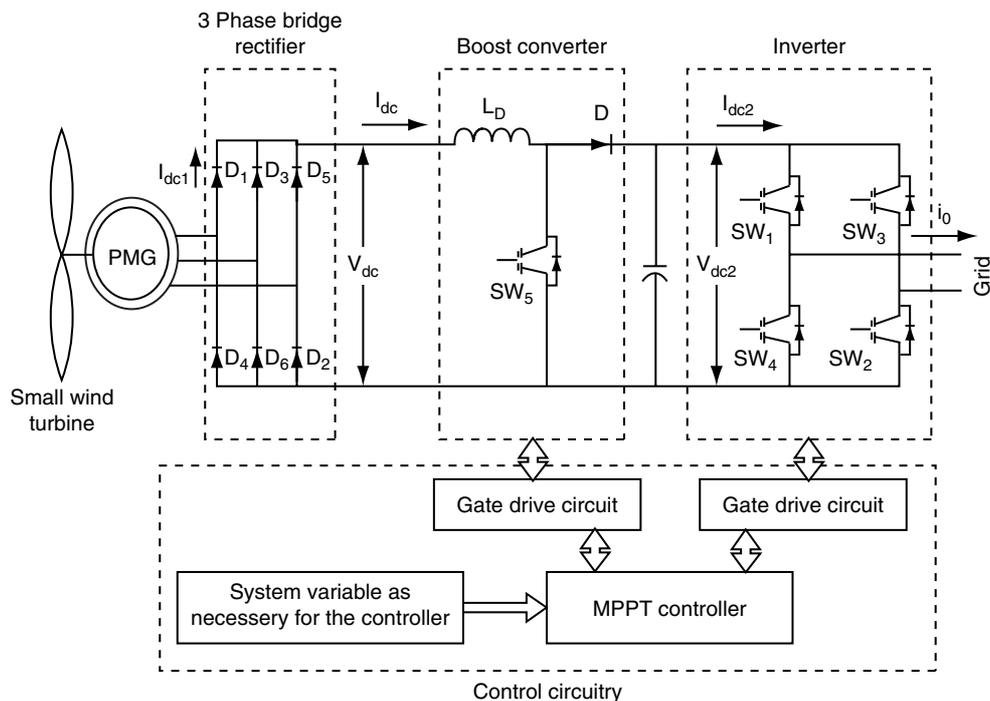
Figure 1: A PMG-based small wind turbine system.
