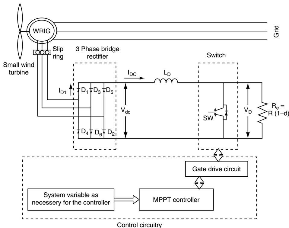
Figure 2: A WRIG-based small wind turbine systems.
