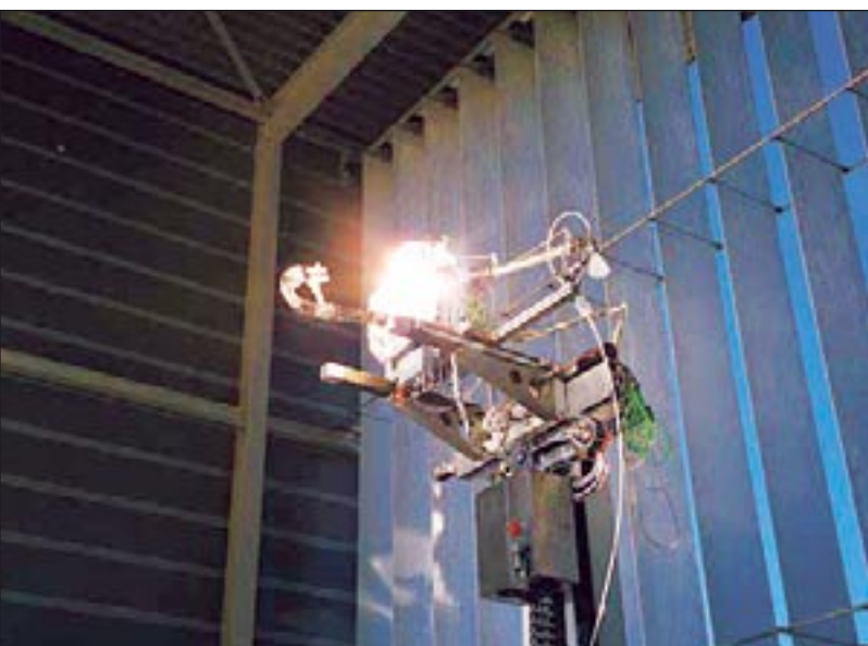
The solar chemical reactor features a vortex flow of methane confined to a cavity-receiver and laden with carbon particles. The source of high-temperature energy is concentrated sunlight. The chemical products are hydrogen and carbon nanofilaments. A schematic view is shown above, while the picture on the left shows the reactor installed in the PSI solar furnace.
